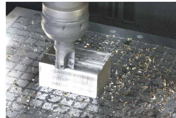
Example 1: Tool model: EMR C32-5R35-150 Z3 Feed: 200, blade: SanlingR5
