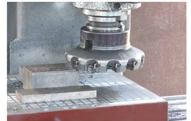
Example 2: Tool model: SE45 50-22 Z4 Feed: 200, blade: Sekt1204
